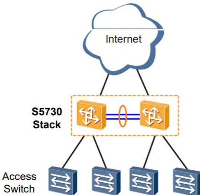
Other than that, the S5730-SI switches can be used as the core switches of a small-sized enterprise campus network, which have powerful aggregation and routing capabilities. The S5730-SI switches use iStack to ensure high reliability. The switches provide various access control policies to achieve centralized user management and simplify configuration.
