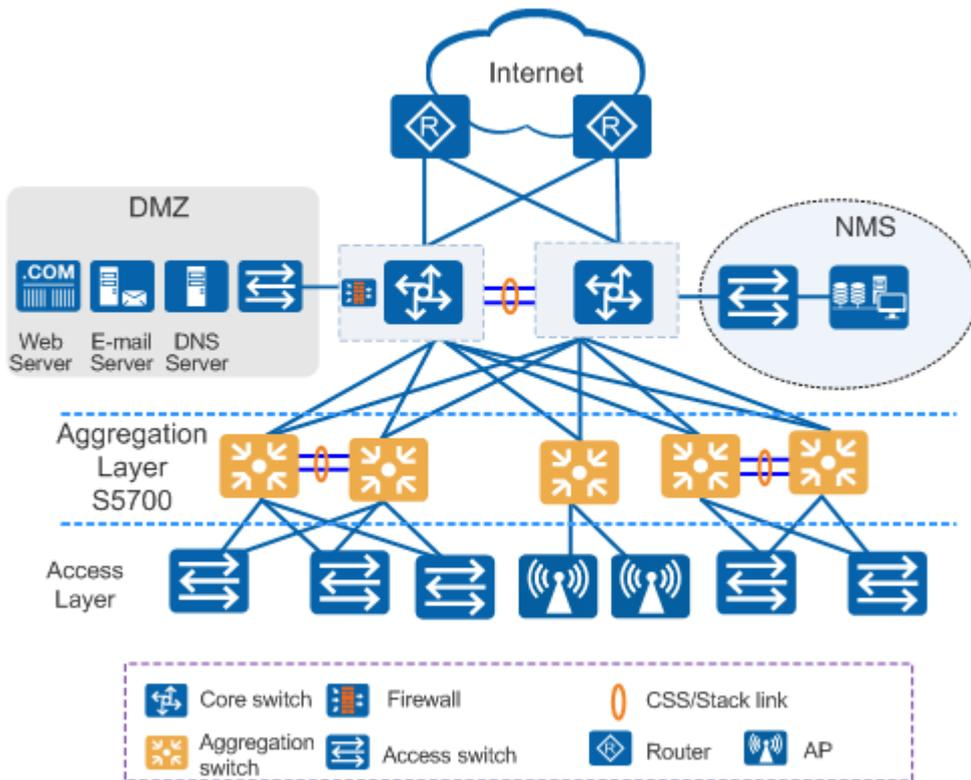
On an enterprise network or campus network, the S5730-SI switches connect to access switches through gigabit or 10 gigabit interfaces, provide high performance and large switching capacity, and connect to core switches through 10 gigabit optical interfaces. The network provides 10 Gbit/s rate for the backbone layer and 100 Mbit/s access rate for terminals, meeting requirements for high bandwidth and multi-service.
